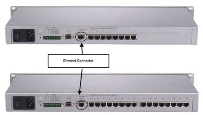
Figure 2.10: Ethernet Connector of EDG-4508R+/4516R+
